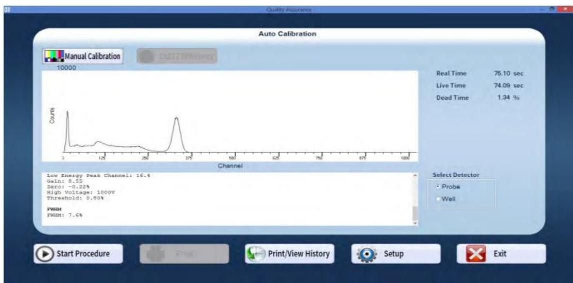
Figure 5: Cs-137 Spectrum in Auto Calibration Process
