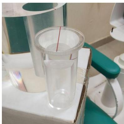
(b) Inner Insert for vial placement
